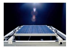
No module leaves our production facilities without meeting strict electrical and optical criteria during the final inspection. Apart from performing routine tests during the production process, we regularly remove modules from series production and check them in our own module testing center. In order to achieve certification to IEC standards 61215 and 61730, the test routines are performed by the VDE.
