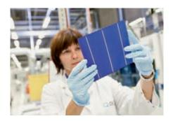
All the materials we use are inspected and assessed against specific parameters before they are allowed to enter the production process. Every cell, for example, is checked for mechanical damage and the quality of its appearance. The glass panels are cleaned and checked for trapped air bubbles and scratches, in order to ensure the greatest possible luminous efficacy.
